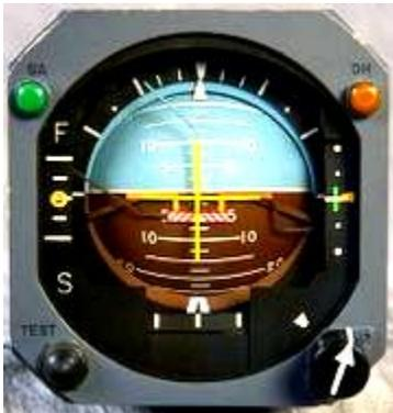
For those of you who don't fly, a horizon indicator is an instrument used in an aircraft to inform the pilot of the orientation of the aircraft relative to earth. It indicates pitch (fore and aft tilt), bank (side to side tilt) and yaw (left to right and right to left). It is displayed like a ball, colored blue on top, dark on the bottom – with a centering line going across it. If the centering line is in the blue, you are climbing. If it is
